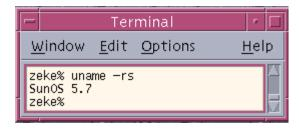
Figure 1.1 An example of the *uname* command usage to find out the name and version of the operating system.
